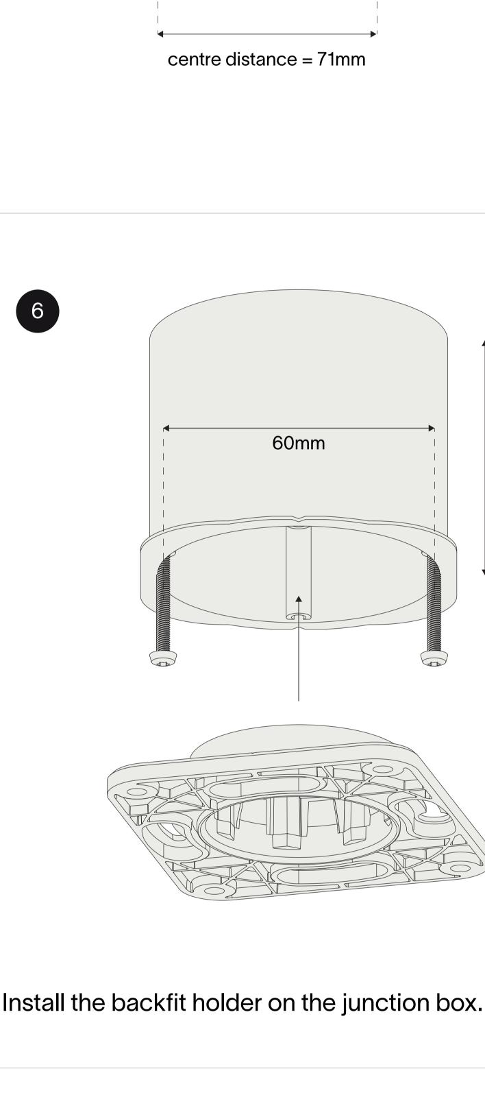
rond 3.0 socket Click the socket in the holder to make alignment easier. max length < panel thickness
